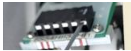
Fig. Disconnecting of cables
