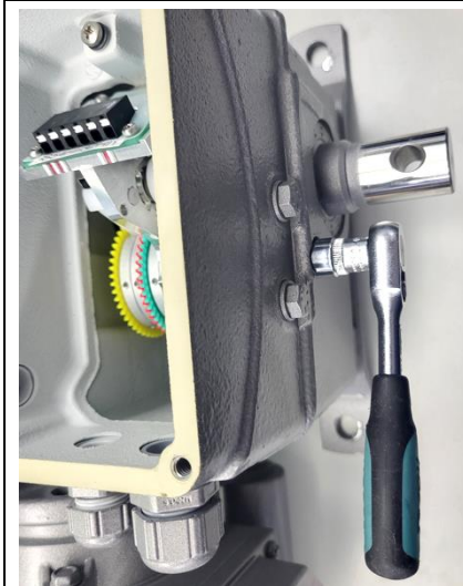
Abb. Disassembling of the fixing screw of limit switch unit
